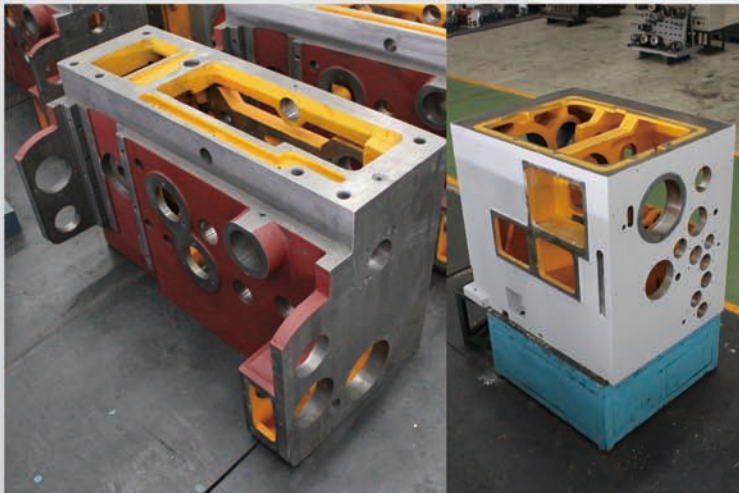
Slide box and headstock The main basic parts are integrally cast with resin sand, with artificial aging treatment and excellent stability of the whole machine
