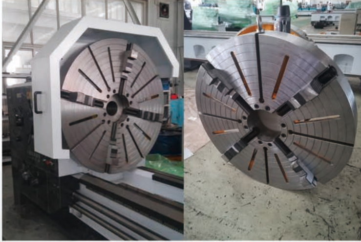
Chuck protection and four-jaw chuck Prevent machine tool operators from being injured and equipment damage
