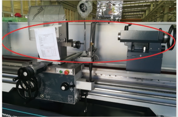
Rear protection Prevent cooling water splashing and iron filings collection
