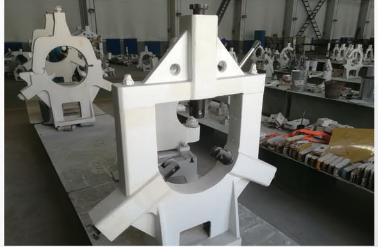
Center frame Standard. Open center frame, stable workpiece rotation
