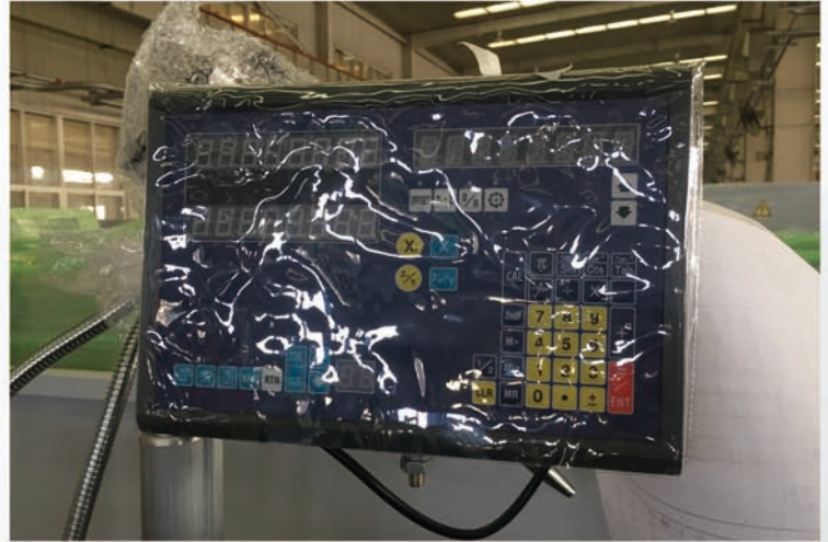
Digital display (DRO) X-axis Y-axis travel is equipped with digital display (precision 0.001)
