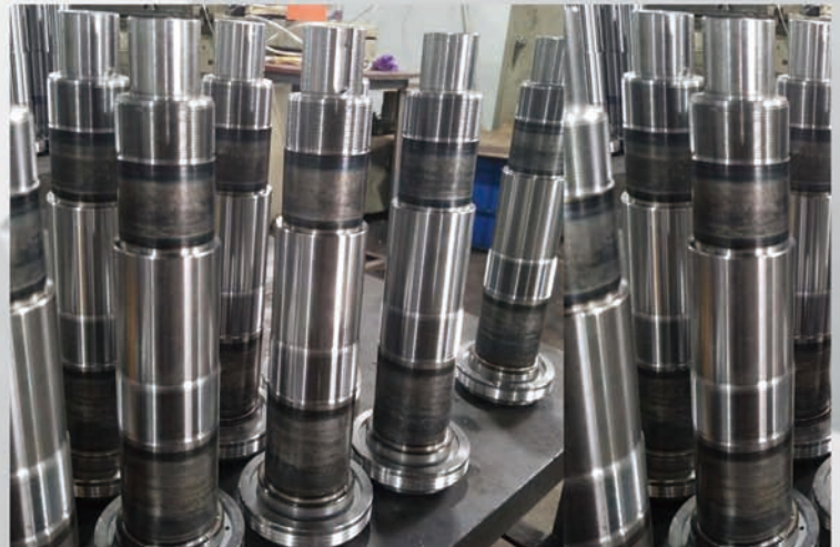
Spindle The operation is convenient and flexible, the main shaft system adopts three-point support, the front and rear bearings have high precision, and the rigidity is strong. The braking and positive and negative changes of the main shaft are hydraulically controlled, and the braking is sensitive and reliable.
