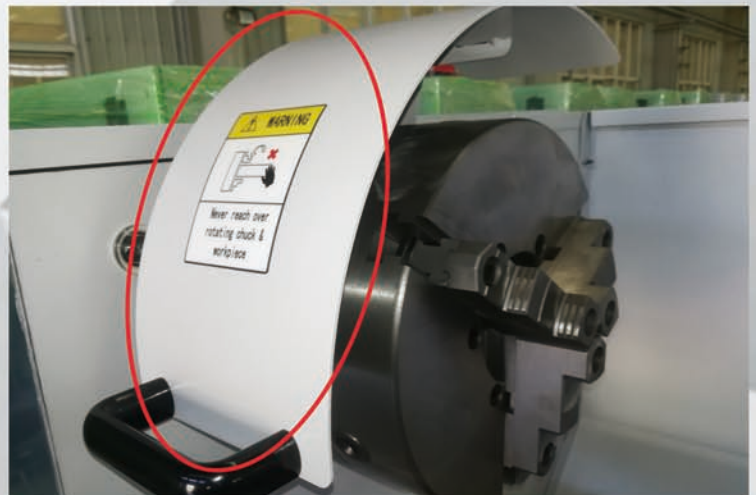
Chuck protection When the protection is closed, the machine runs. When the protection is open, the machine stops.
